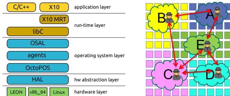
**Figure 4.16:** iRTSS Architecture. Left the overall layered organisation of iRTSS (blue), right the structure of the distributed agent system.
